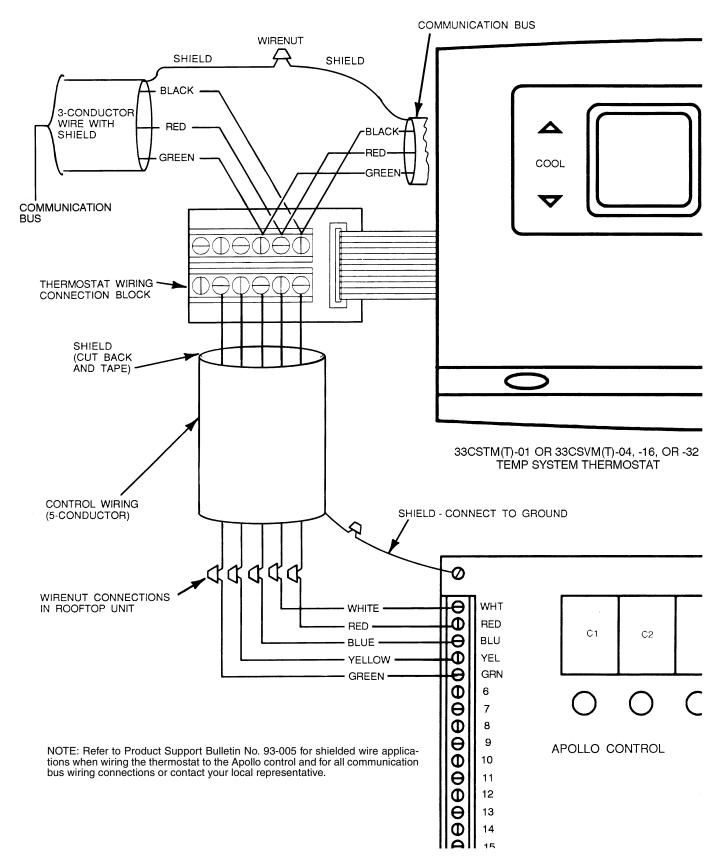
Fig. 6 — Thermostat and Apollo Control Wiring
